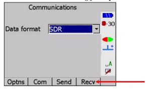
17. Back to *SOKKIA Link*, click **Data Send**. When finished, a window box will appear on computer and instrument, click **OK**.
